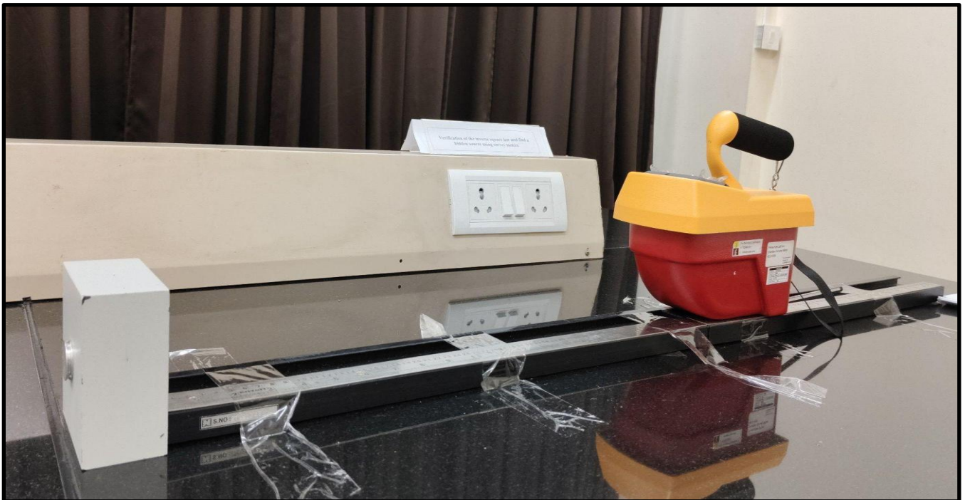
Fig. Setup for Verification of Inverse Square Law
